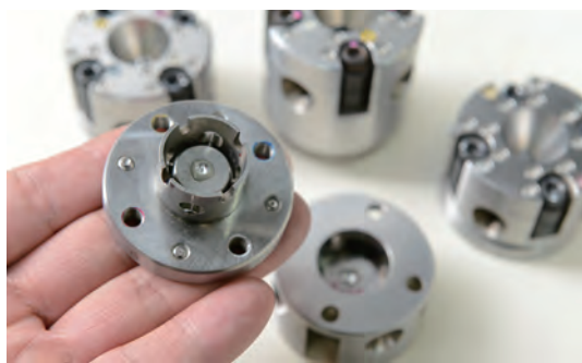
Fig. 3 Diamond anvil cell that reproduces an ultra-high pressure state
