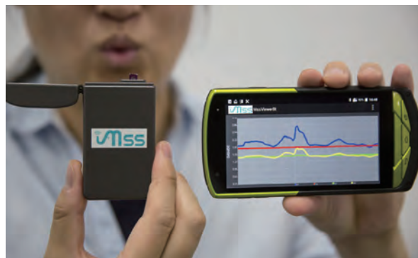
Fig. 6 Application as a mobile olfactory sensor device for monitoring health conditions by analyzing exhaled breath.
