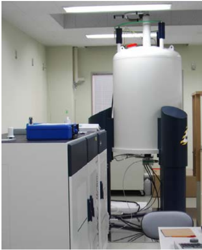
The 11.7T MRI system at high performance bioimaging research facility, Osaka University (Left). Sample imaging of mouse head using the 11.7T MRI (Brucker)
