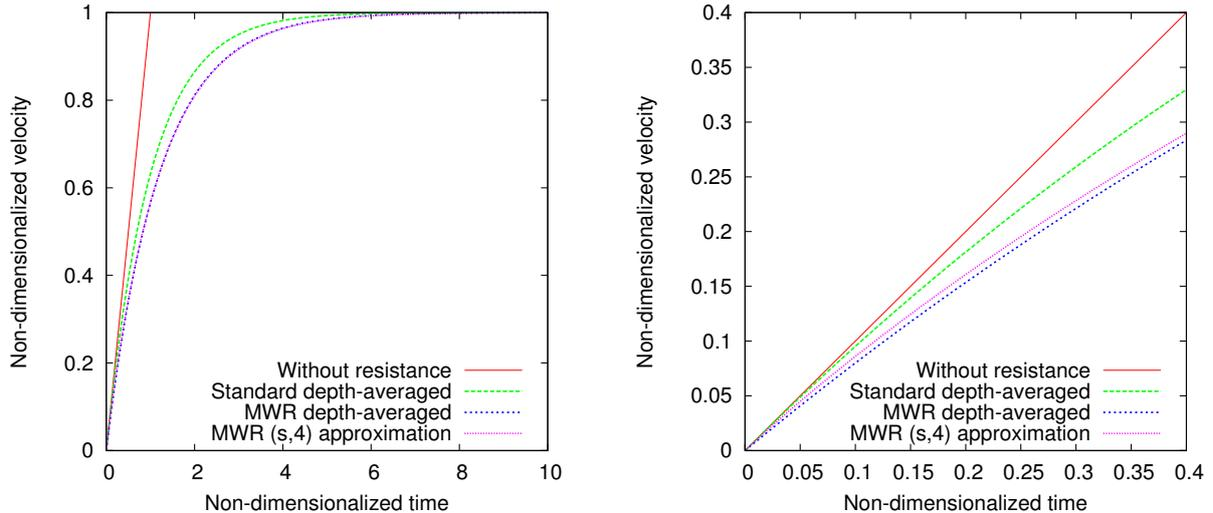
Figure 6: Comparison of the time evolution of the depth-averaged velocity between the standard slab model, the slab model derived with the MWR, and the fourth-order expansion in the sine-basis. The latter gives results that are visually indistinguishable from the exact solution.
