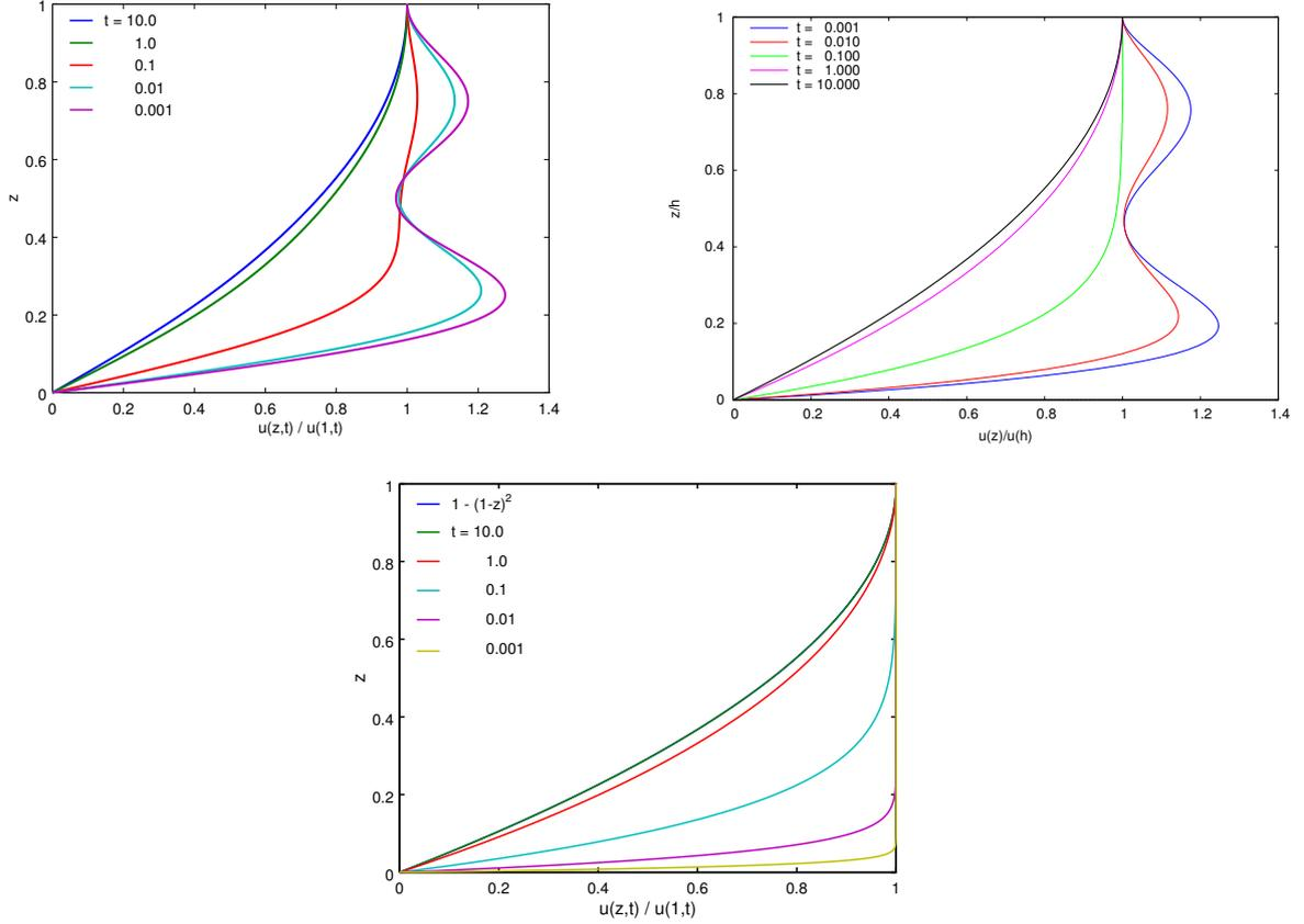
Figure 7: Evolution of the normalized profile function with time for the fourth-order approximations in the sine-basis (left panel) and polynomial basis (right panel). For comparison, the bottom panel shows the exact solution. For  $t = 10$ , it coincides visually with the asymptotic parabolic profile. For  $t < 0.1$ , neither approximation is capable of reproducing the bluntness of the exact solution, but for  $t \geq 0.1$ , the agreement is quite good.
