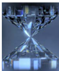
Fig.1. High-pressure device called diamond-anvil cell (DAC)
