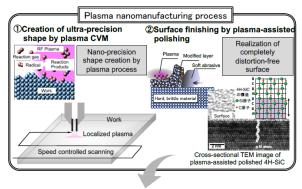
Innovation in manufacturing technology by building a completely distortion-free processing system
