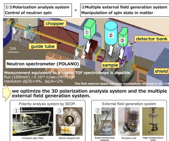
The high-energy neutron spectrometer POLANO installed at J-PARC, the SEOP polarization analysis system and the multiple external field generation system introduced in this study.
