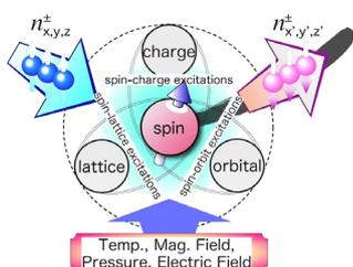
Conceptual diagram of research content. Detailed spin information is extracted from the multi-degree-of-freedom composite excitation of electrons using polarized neutrons. By applying an external field to the sample, a change in the spin state is induced to obtain more detailed information.
