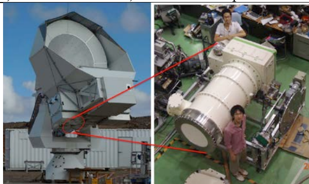
Figure 1 The radio telescope we currently use for the POLARBEAR project (left), and the POLARBEAR-2 receiver system in preparation (right).
