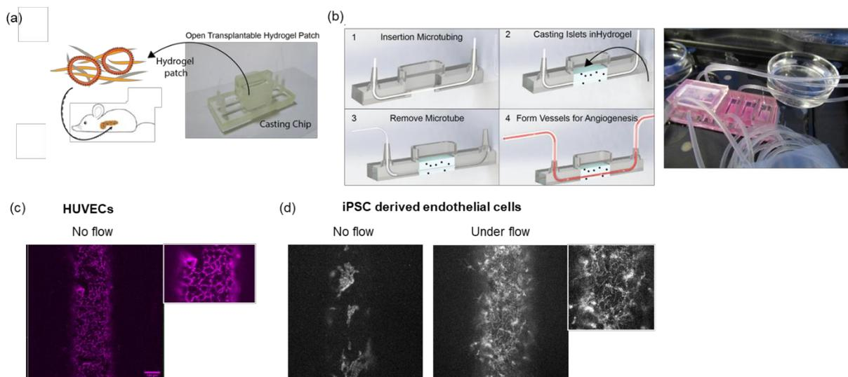
Figure 3. (a) Possible application of lumen chip. (b) Design principle to create lumen formation in casting gel using microtube. (c,d) We cultured HUVECS (c) and iPSC-derived endothelial cells (d) in the lumen and cells were stained with VE-cadherin antibody.
