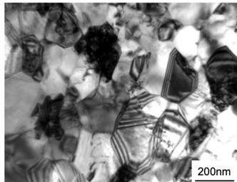
Fig.2 TEM image of a Bulk Nanostructured Metal
