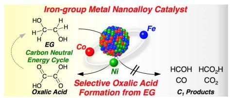
Fig. 1.12. CO<sub>2</sub>-free power generation by selective fuel oxidation with iron-group nanoalloy catalysts.
