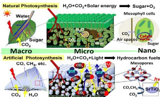
Fig. 10. Schematic illustration and comparison of the structure and key processes in (top) natural photosynthetic system and (bottom) artificial photosynthetic system.
