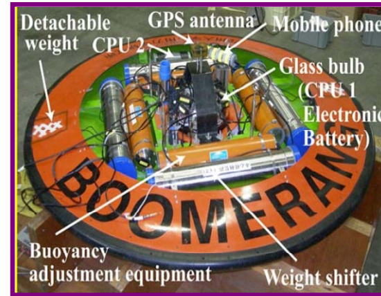
Fig. 9b. Underwater vehicle for CO 2 monitoring in the deep ocean
