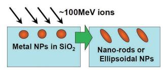
Fig. 2. The phenomenon called "shape elongation of embedded NPs" is schematically depicted. The rectangles show the cross-sections of the  $SiO_2$  matrix including NPs. Under SHI irradiation, spherical NPs deform to nano-rods.
