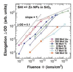
Fig. 3. Fluence dependences of the shape elongation of Zn NPs embedded in silica. The samples were irradiated with a wide variety of ion species and energies, ranging from 1.7 MeV Si<sup>+</sup> to 200 MeV Au<sup>13+</sup>, using three different accelerator facilities in Japan and India [1].
