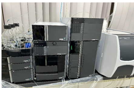
Figure 14: Size exclusion chromatography with total carbon analyzer
