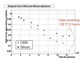
It is a significant step to confirm that we can use the CIGS semiconductor as a particle detector with a recovery feature for radiation damage. A paper is in preparation.
