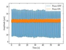
tried to mitigate the vertical vibration using an actuator (in open loop mode) and successfully demonstrated it. Next year, we aim to develop a feedback control circuit and control all the six degrees of freedom.
