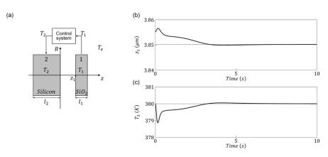
As a preliminary study, we consider a system consisting of two SiO<sub>2</sub> and Si parallel plates interacting through Casimir force and thermal emission. The temperature T<sub>2</sub> of the silicon plate is adjustable, and the ambient temperature is
