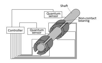
the shaft. Based on the information, the temperature of each piece is adjusted so that the shaft has no contact with the bearings.
