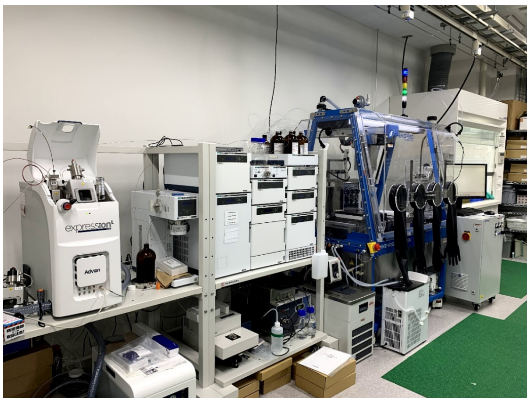
Figure. Automated chemical synthesizer designed for organic synthesis, which can quickly validate new chemical reactions, at ICReDD Mix-Lab
