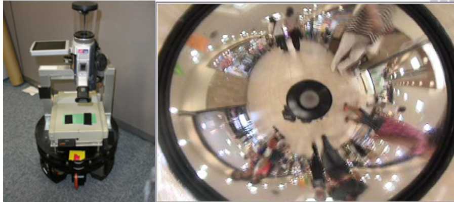
Figure 2: A mobile robot (left) was used to gather ODVS image (right)
