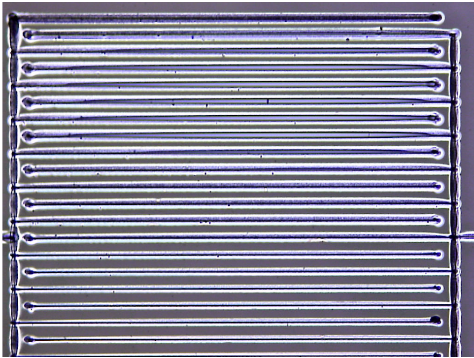
Figure 2. Printed silver interdigitated high aspect ratio walls.
