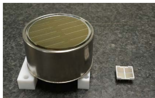
Figure 2 a newly developed sensor (right) and a PMT
