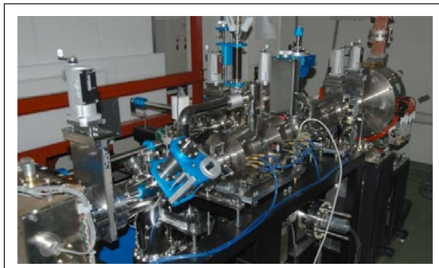
Fig.1 Our time-resolved electron diffractometer
