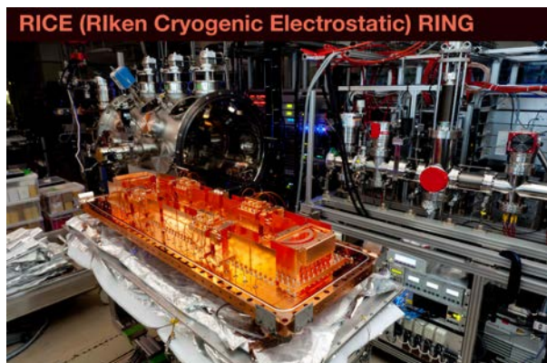
Figure 1 an assembly of the electrodes of the cryogenic electrostatic ion storage ring
