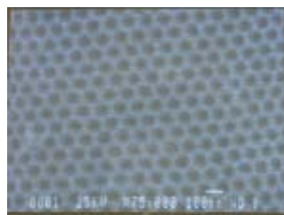
A SEM picture of nanopore array in porous alumina, which is employed in this project.
