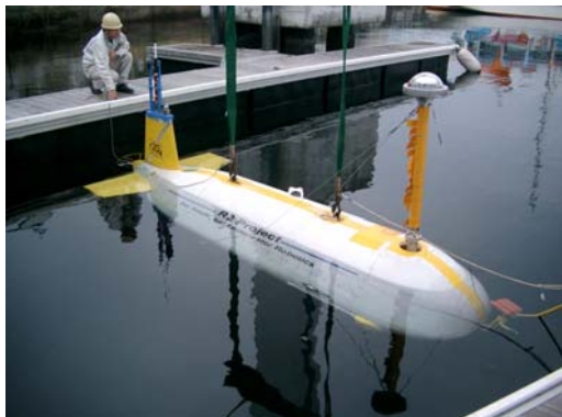
Fig.2 Trial model of the sea surface units installed in the AUV r2D4 for a new generation seafloor geodetic observation technology.
