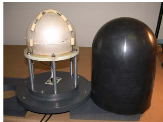
Fig.1 Newly-developed acoustic transducer who has a spherical ceramic oscillator. It gives isotropic feature in phase response.
