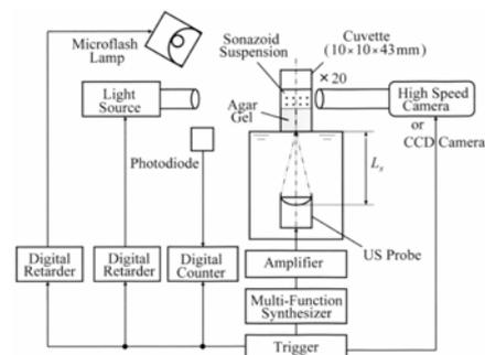
**Figure 1:** Schematic illustration of experimental setup.
