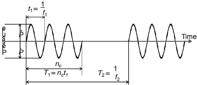
$$DC (\%) = \frac{T_1}{T_2} = n_c \frac{f_2}{f_1}$$
