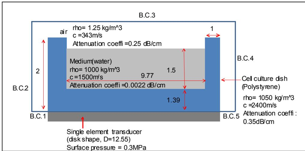
**Figure 3.** Boundary conditions of theoretical model.
