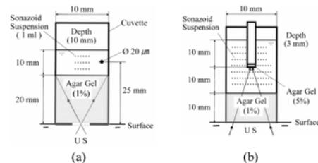
**Figure 2:** Two types of test section, (a) Case A and (b) Case B.
