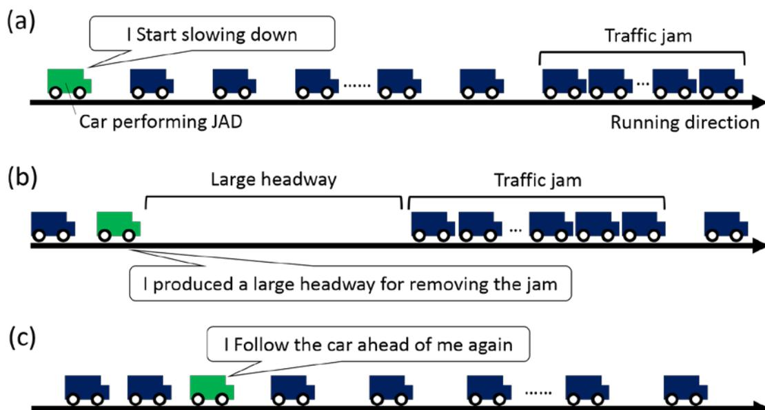
Figure 1: Schematic views of JAD. (a) A traffic jam is moving from right to left direction. The car performing JAD starts slowing down. (b) It produced a large headway. Then, the jam is removed. (c) After disappearance of the jam, it follows the car ahead of it again.
