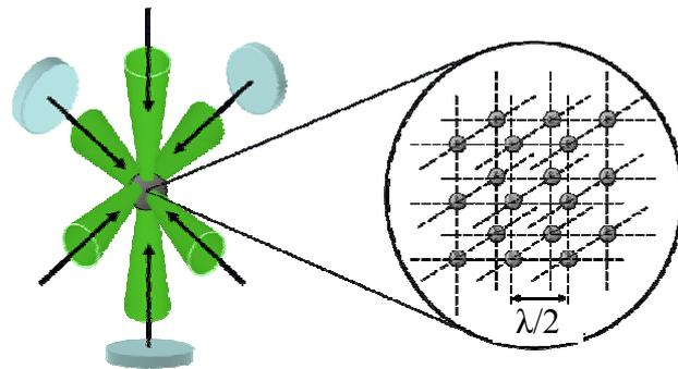
for atoms produced by a standing wave of laser light depicted above. Two internal quantum states in each atom loaded in one optical lattice site is regarded as a fundamental quantum bit in this quantum computer, and an individual addressing can be possible by a spectral addressing under a magnetic field gradient, the principle of which is essentially the same as the magnetic resonance imaging.
