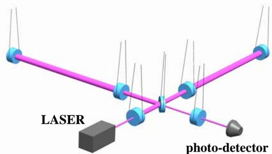
Fig.1: Schematic of a gravitational-wave detector.
