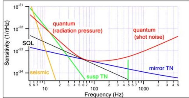
Fig.2: A typical noise budget of a second-generation gravitational-wave detector.
